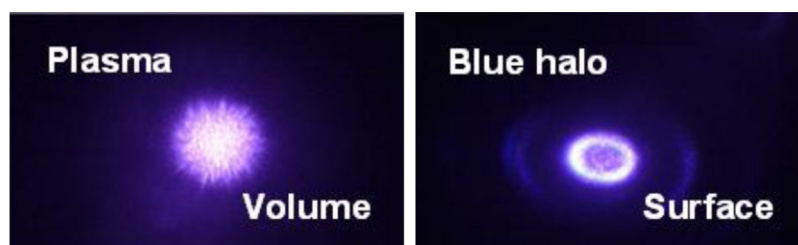
Fig. 5. Images of the laser-induced plasma, when the focus is within the bulk volume of the sample or at the sample surface.
