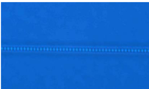
Fig. 7. Demonstration of control degree of laser repetition rate and sample velocity allowing definition of highly controllable index modulation points.
